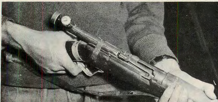
Simple tools and common junk were all Mau Mau gunsmiths needed to make weapons. This one fired .303 British service cartridges.
